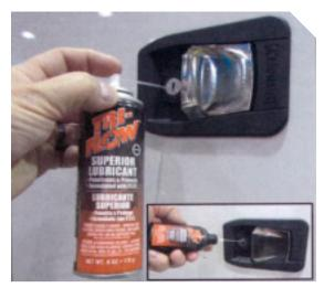
**B. Lubricate Door Lock Cylinders**
